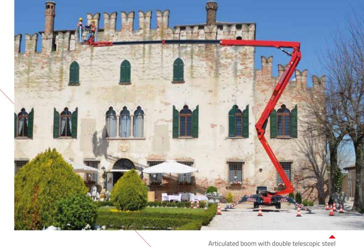
boom, in Domex® 700 with wall thickness from 3 to 5mm for max service life and stiffness.
