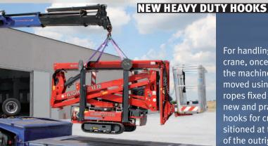
For handling by crane, once closed, the machine can be moved using ropes fixed on these new and practical hooks for cranes positioned at the end of the outriggers.
