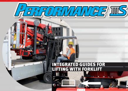
Lightlift 17.75 PERFORMANCE a forklift can be used to transport the machine. This system is very useful to move the machine on the construction site and to load and unload.
