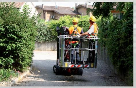
The innovative Auto2Speed traction system allows the machine to reach an optimal translation speed of 3.6km/h, to move quickly from one place to another on the construction site. Furthermore. thanks to the inclination control, the machine automatically decelerates in extreme conditions to enhance operator's safety.
