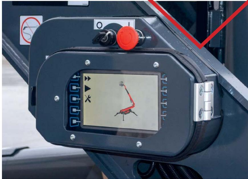
▲ LCD smart vision panel for ground controls
