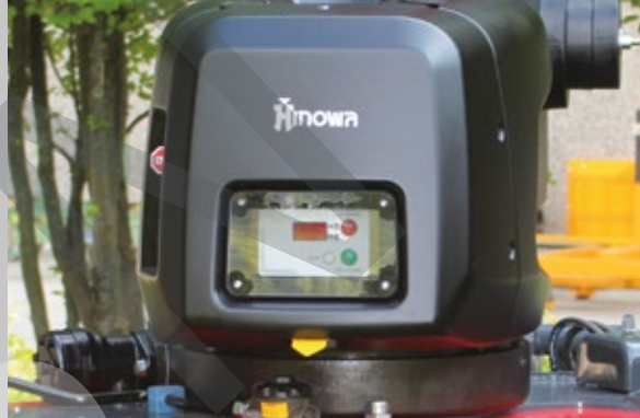
Battery charger and display indicating the charge status of the TeleCrawler13N
