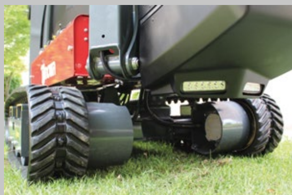
LED front and rear working lights
