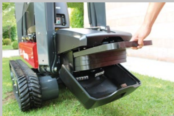
Stabilization plates holder with locker
