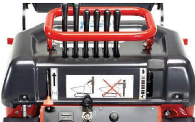
The control panel is in front of the operator and is comfortable and user-friendly. All control levers are easy to reach and a grab handle bar secures the operator while working.
