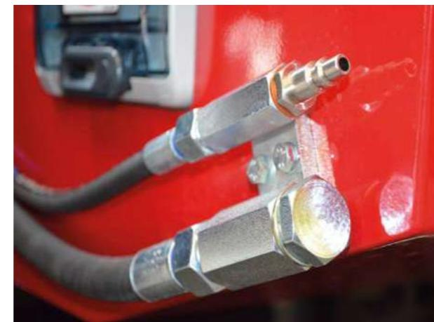
**Ø1/4" Auxiliary line to the basket allowing to use different working tools.** Double auxiliary line ( $\varnothing 1/4"$  +  $\varnothing 1/2"$ ) on models LL13.70, LL15.70, LL18.80, LL20.10MK3 and LL26.14 MK2.
