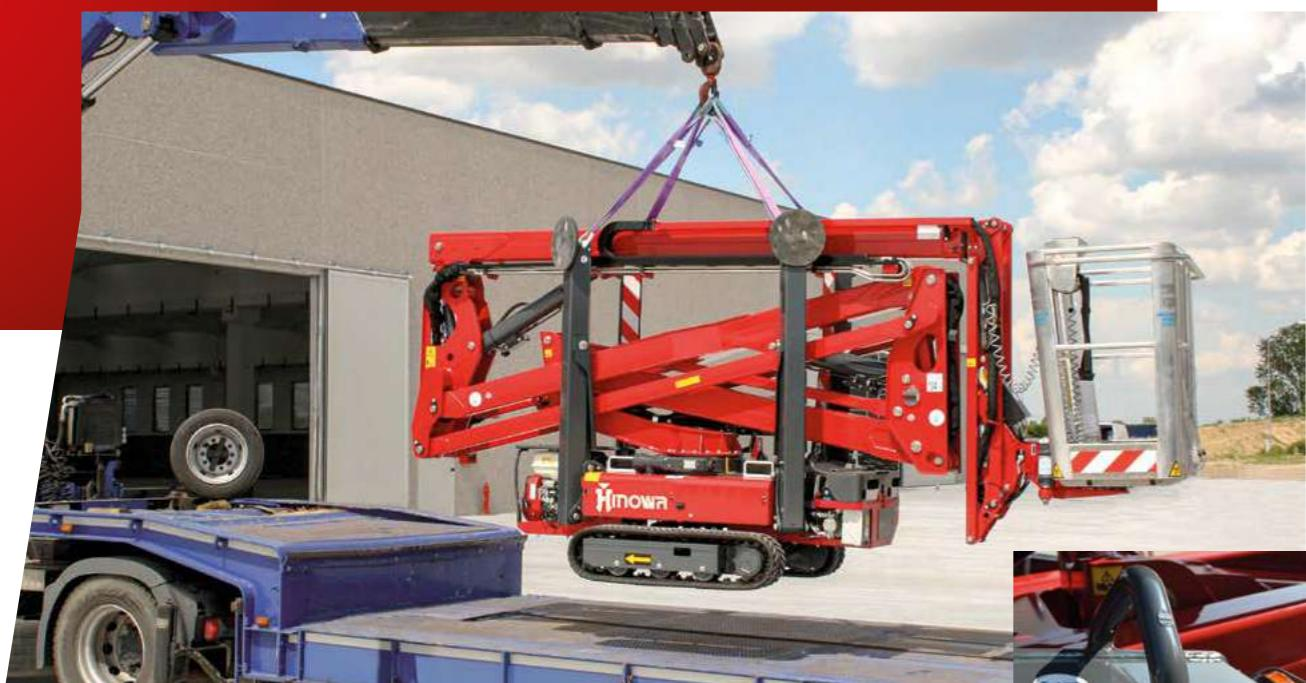
**Heavy Duty lifting hooks** on outriggers for positioning with crane.
