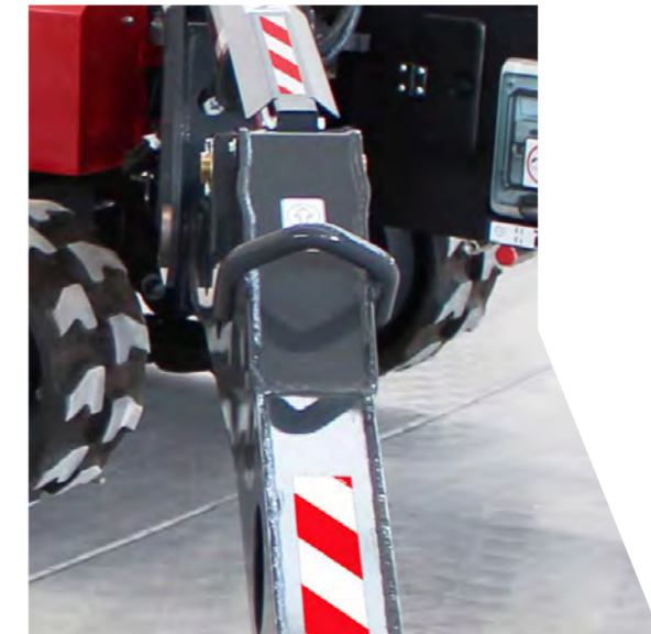
Heavy Duty lifting hooks on outriggers for positioning with crane.
