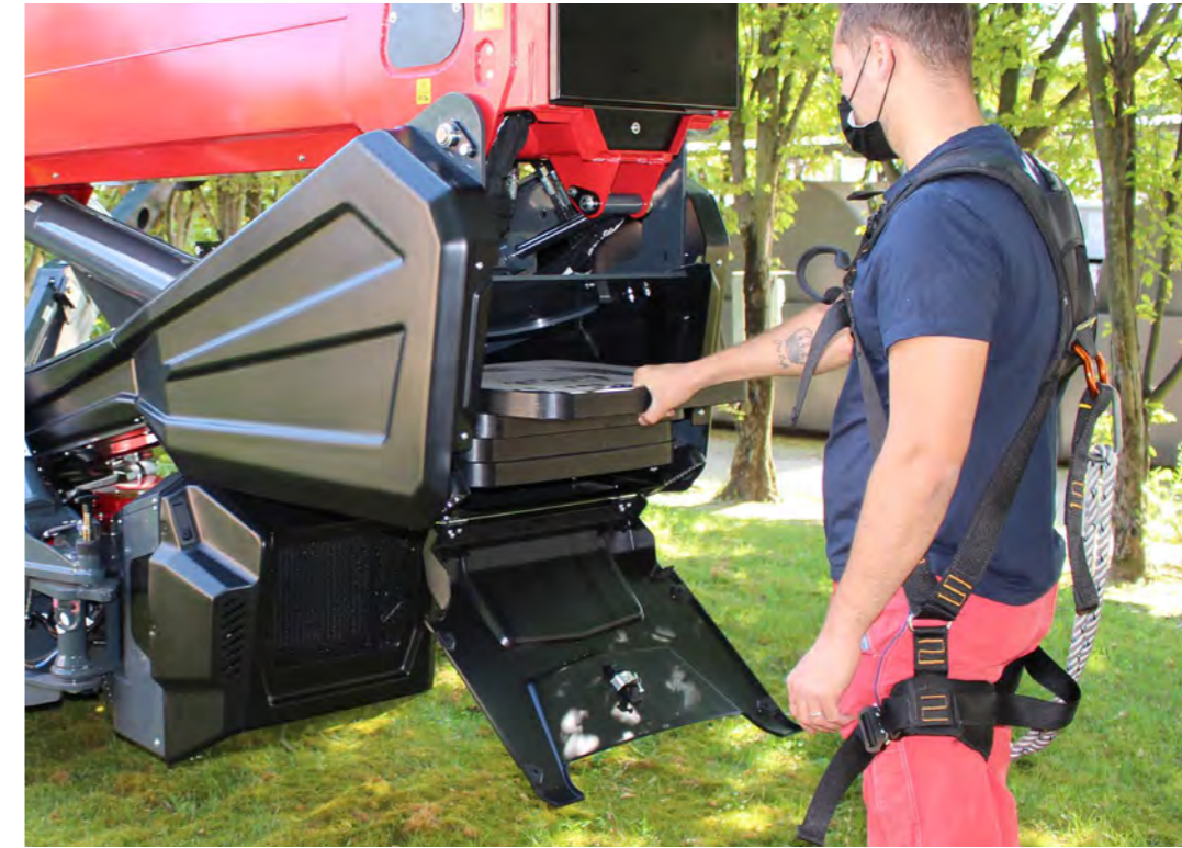
Built-in container with key for stabiliser plates. (In the TC22 Lithium version, the container is located in the bottom part where the diesel engine is normally housed).
