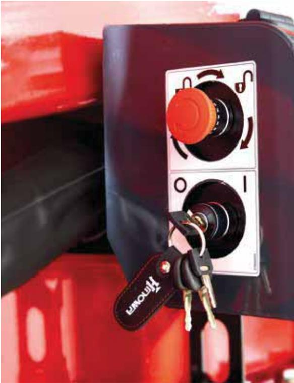
▼ Simplified ignition system with a **single key**.
