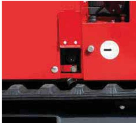
▼ **Auxiliary connector** for external devices, telematics and fleet tracking.
