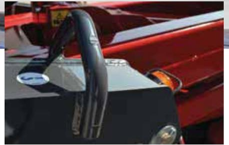
▼ Heavy Duty lifting hooks on outriggers for positioning with crane.
