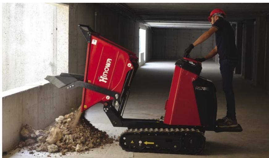
**CON UNA LARGHEZZA DEI CINGOLI DI 180 MM E UN PESO SENZA OPERATORE DI 590 KG, L’HS701E LITHIUM OFFRE UNA CAPACITÀ MASSIMA NOMINALE DI 0,34 M<sup>3</sup>**
